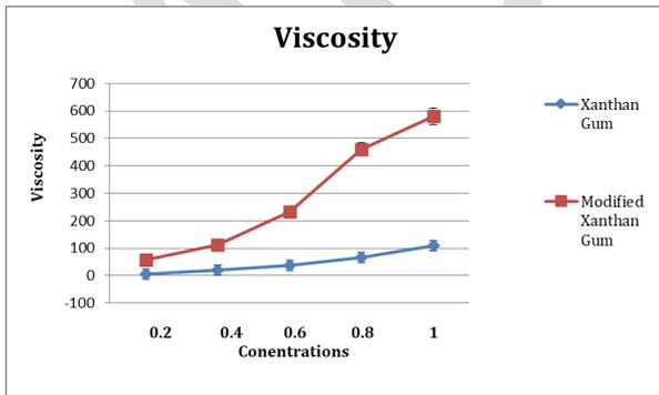
Fig. 9: Comparative viscosity study of Xanthan gum and Modified Xanthan gum. Illustration values are the mean of three experiments  $\pm$ SD.
