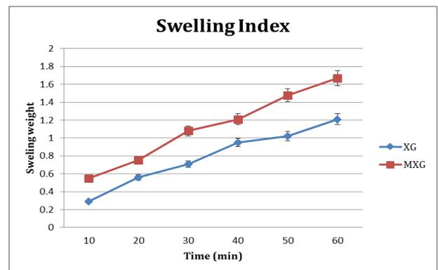
Fig.10: Swelling behavior of Xanthan gum and Modified xanthan gum in simulated saliva solution, Illustration values are the mean of three experiments  $\pm$ SD.
