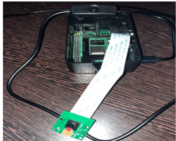
Figure (22): Raspberry Pi connected to Pi camera.
