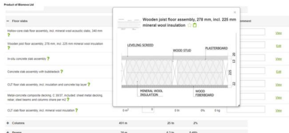
Figure (4): wooden joist floor 278mm, inci 225mm mineral wool insulation.
