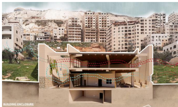
Figure (5): Demonstrating natural cooling using heat sinks and ventilated enclosures. By Julien Yray, 2023.
