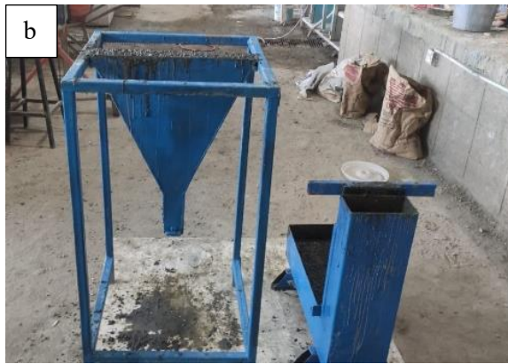
Figure (2): Fresh material test, (a) passing ability, (b) flowability.
