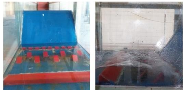
Figure (4): The first modified model of redistribution of baffle blocks within the laboratory channel before and during operation.
