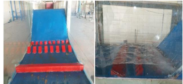
Figure (3): Standard model inside the laboratory channel before and during operation.
