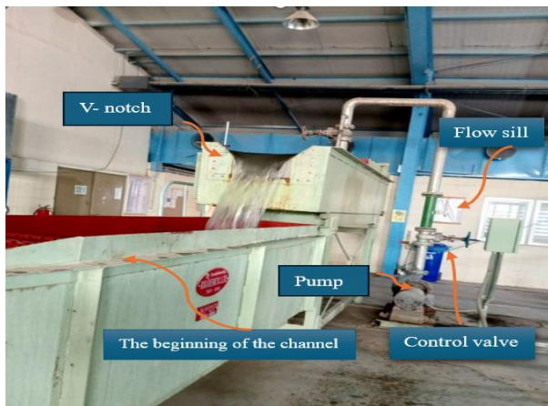
Figure (2): Part of the laboratory channel used for carrying out physical experiments, showing a partial view of the details of the internal structure
