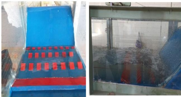
Figure (6): The third modified model with a second row of baffle blocks added inside the laboratory channel before and during operation.
