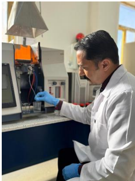
Figure (3): Sampling analyses using flame atomic absorption spectrometry.
