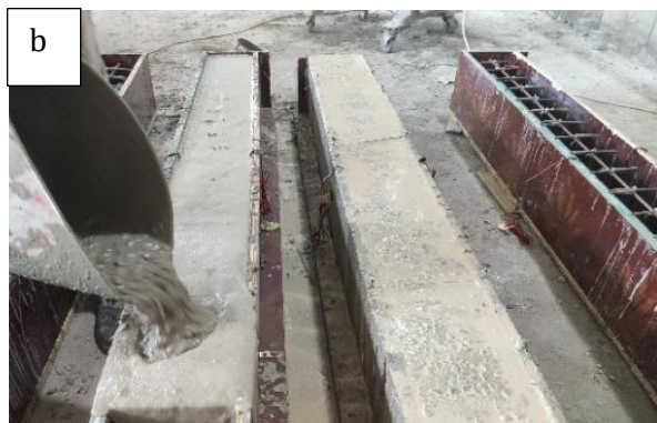
Figure (4): Details of experimental work, (a) reinforcement bars (b) concrete pouring.
