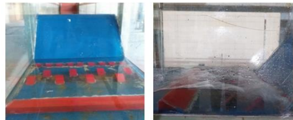
Figure (4): The first modified model of redistribution of baffle blocks within the laboratory channel before and during operation.
