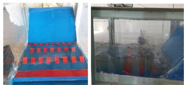
Figure (6): The third modified model with a second row of baffle blocks added inside the laboratory channel before and during operation.
