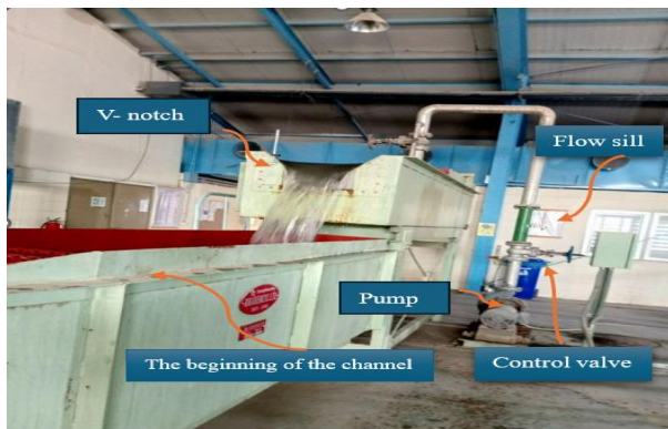
Figure (2): Part of the laboratory channel used for carrying out physical experiments, showing a partial view of the details of the internal structure
