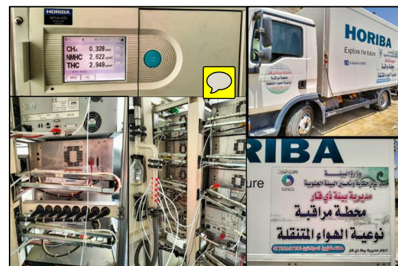
Figure (2): Calibration method and comparison of results with the vehicle designated for measuring gases.
