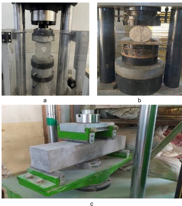
Figure (4): Experimental Tests Conducted: (a) Compressive Strength, (b) Indirect Tensile Strength, (c) Flexural Strength.
