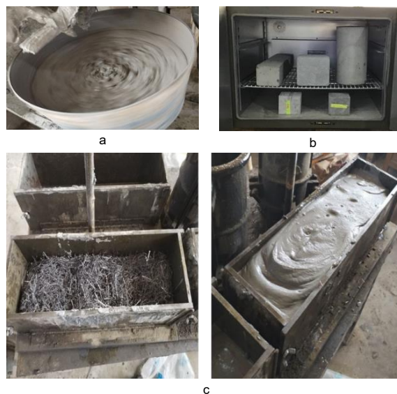
Figure (2): a) The mixer used to prepare bauxite-concrete slurry, b) Samples during exposure to the curing process, c) Bauxite SIFCON concrete cast by (immersed technique)
