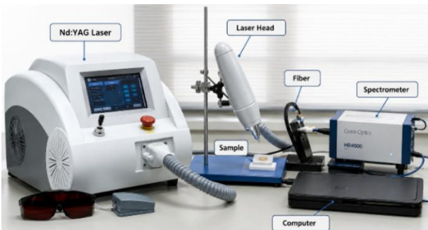
Experimental setup for LIBS analysis of nail samples using an Nd: YAG laser system. The laser -induced plasma emission is collected via an optical fiber and analyzed by a high-resolution spectrometer. The system is controlled by dedicated software.
