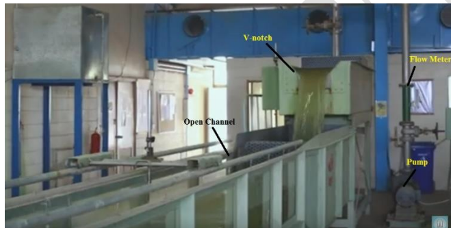
Figure (2): The open channel V-notch weir.
